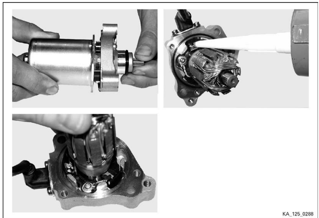
Figure 圖 7.16: Electric starter disassembly 拆解啟動電機總成
